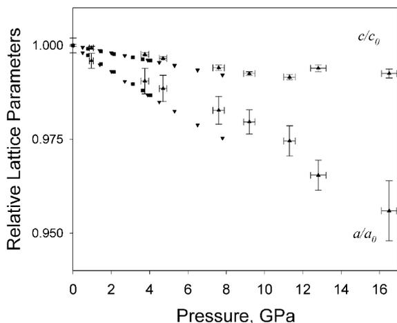
Fig. 3. Variation of relative lattice parameters ( $a/a_0$  and  $c/c_0$ ) of nano-anatase with pressure (triangles) in comparison with data for polycrystalline bulk material (inverted triangles, from Ref. [18]) and for a single crystal (squares, from Ref. [15]).
