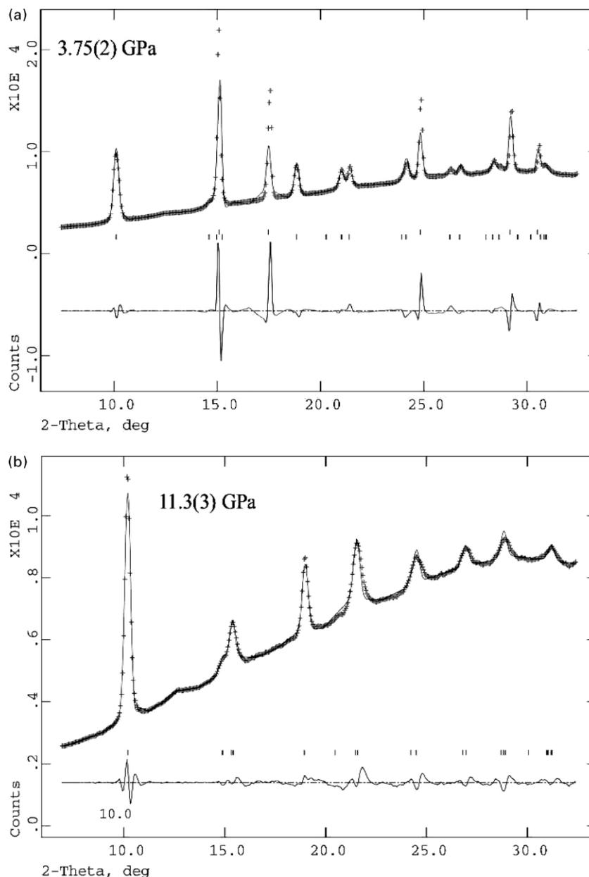
Fig. 2. Examples of the full-profile refinement of the X-ray diffraction data collected: (a) at 3.75(2) GPa and (b) at 11.3(3) GPa. The upper ticks represent Au, and the lower ticks—anatase. Deviation of the refined intensities from those experimentally observed for gold diffraction lines at 3.75 GPa are related to the complex preferred orientation on gold wire.
