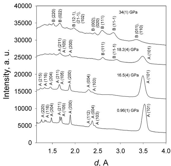
Fig. 1. Representative powder X-ray diffraction patterns obtained from compressed nanocrystalline anatase. Reflections marked A originate from anatase, and those marked B from baddeleyite-TiO<sub>2</sub>.
