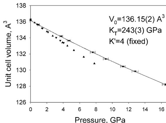
Fig. 4. Room-temperature pressure–volume data of nano-anatase (circles) compared with data from polycrystalline (triangles, from Ref. [18]) and single crystal (inverted triangle, from Ref. [15]) anatase.
