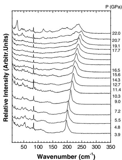
**Figure 6.** Evolution of  $\text{Cs}_2\text{HgBr}_4$  Raman spectra with applied pressure between 3.9 and 22.0 GPa in zone C. This run was performed with argon as the pressure-transmitting medium. The line at  $75\text{ cm}^{-1}$  is a plasma line from the laser.
