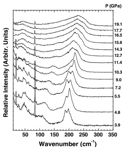
**Figure 4.** Evolution of  $\text{Cs}_2\text{HgBr}_4$  Raman spectra with applied pressure between 3.9 and 19.1 GPa in zone A. This run was performed with argon as the pressure-transmitting medium. The line at  $75\text{ cm}^{-1}$  is a plasma line from the laser.
