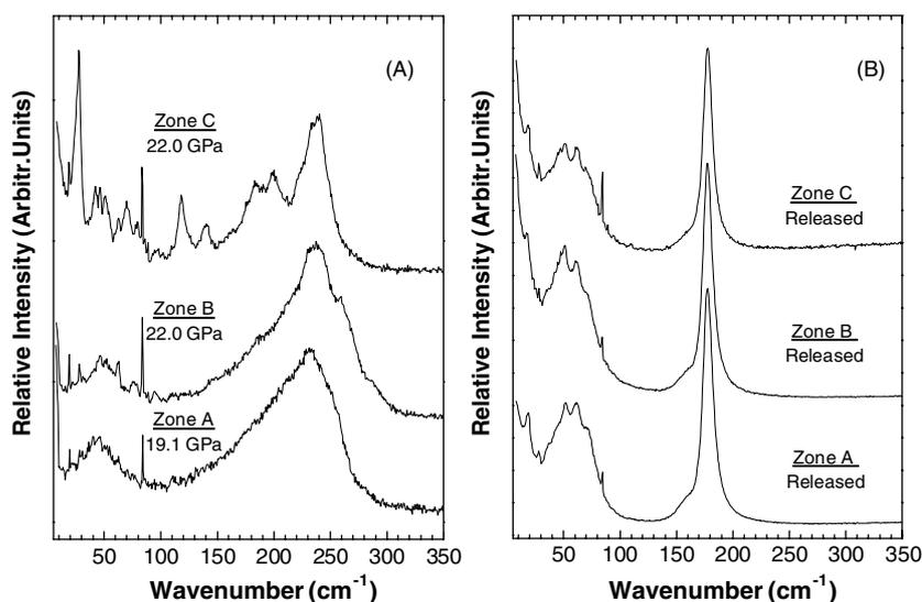
**Figure 7.** Comparison of  $\text{Cs}_2\text{HgBr}_4$  Raman spectra obtained in the zones A, B, and C defined in figure 3. (A) Spectra recorded at the highest pressure. (B) Spectra recorded after decompression. The line at  $75\text{ cm}^{-1}$  is a plasma line from the laser.
