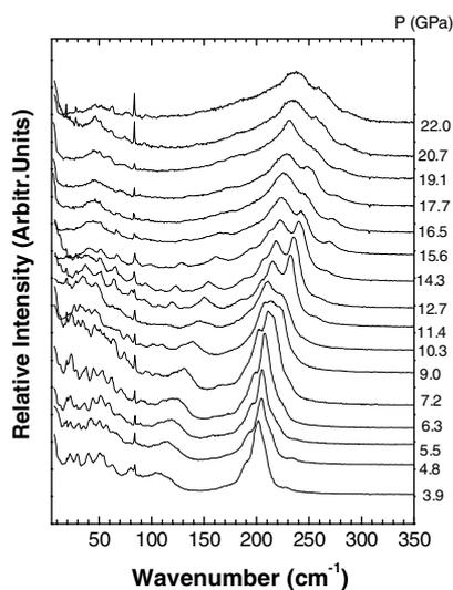
**Figure 5.** Evolution of  $\text{Cs}_2\text{HgBr}_4$  Raman spectra with applied pressure between 3.9 and 22.0 GPa in zone B. This run was performed with argon as the pressure-transmitting medium. The line at  $75\text{ cm}^{-1}$  is a plasma line from the laser.
