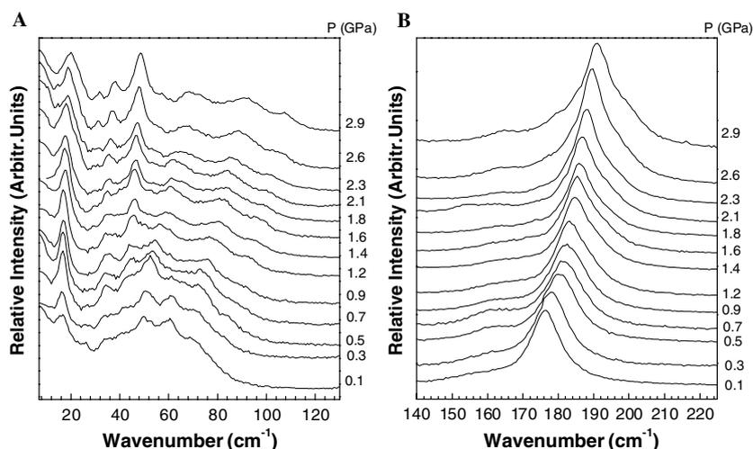
**Figure 1.** Evolution of Cs<sub>2</sub>HgBr<sub>4</sub> Raman spectra with applied pressure between 0.1 and 2.9 GPa. (A) Lattice modes and bending internal modes; (B) stretching internal modes. This run was performed without any pressure-transmitting medium.
