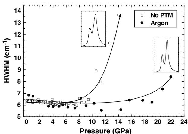
**Figure 8.** Half-width at half maximum (HWHM) evolution of the luminescence ruby line in both experiments. Open squares: without any pressure-transmitting medium; circles: argon as the PTM. The lines are guides to the eyes. The two insets show the ruby fluorescence lines at 13.9 GPa during the non-hydrostatic run (no PTM) and at 22.0 during the quasi-hydrostatic run (Ar as the PTM).
