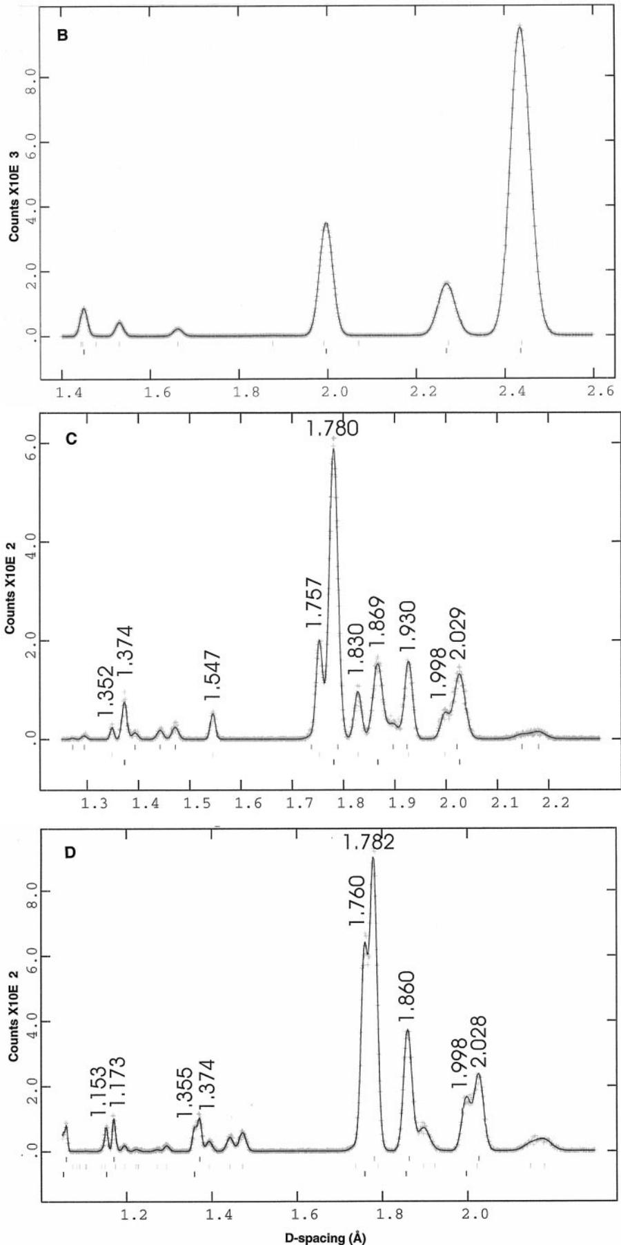
mixture of corundum,  $\epsilon$ -Fe and iron oxide. This line was observed in our previous experiments with iron (23–25) and has been explained as the most intensive (102) dhcp-Fe (double hexagonal close packed) line, which could appear alone in the case of an incomplete transformation from hcp to dhcp structures, or which could be a result of effects of preferred orientation (26).
