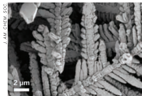
An SEM image displays silver dendrites on aluminum foil.
